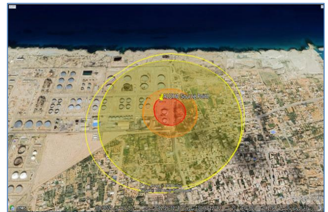
Figure 13: (a) ALOHA blast wave and (b) Goggle earth aerial view threat zones at 10% of the capacity of LPG – 6.
