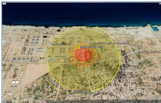
Figure 14: (a) ALOHA blast wave and (b) Google earth aerial view threat zones at 20% of the capacity of LPG – 6.
